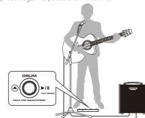
2. If the loop function is active before drum machine, the drum machine will detect the speed of your loop phrase and set the tempo accordingly automatically. If the drum machine is active before loop function, the rhythm tempo will be set at 80BPM and you can change the speed with Smart TAP Tempo function.
