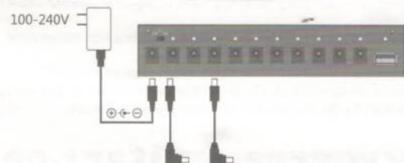
2. If the power adapter is not the original adapter, please make sure the power is 18V 1A with polarity negative internal and positive external. If the adapter does not meet the requirement, please use a polarity conversion cable shown as below.
