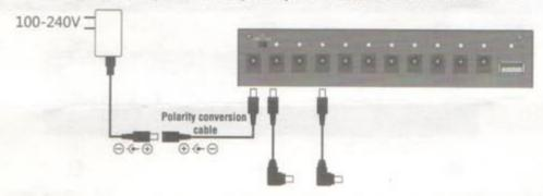
Attention: Please check the polarity of power adapter before using, or it may damage the equipment.
