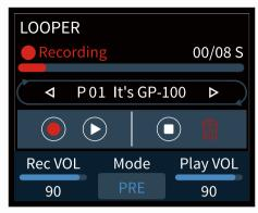
Simultaneously hold two footswitches until the LOOPER menu appears.
