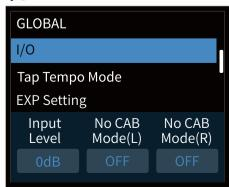
This menu is to set up global input/output settings. Adjust the optimal Input Level for the instrument or other sound source you're using.
