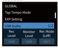
This menu is to set up USB audio settings when using GP-100 as a USB audio interface.
