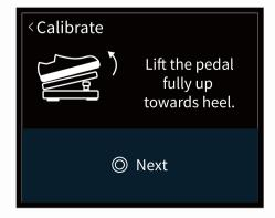
Bring the pedal all the way up (back) and press the PARA button to next step.
