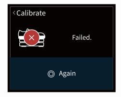
If pedal calibration fails, press the the PARA button to re-calibrate.
