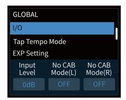
No CAB Mode is for connecting to instrument amplifiers without changing saved presets.
