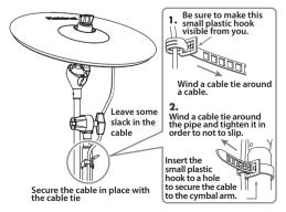
\* Take care to ensure that the cables do not touch the V-Cymbal pads and/ or the stand. A cable touching a V-Cymbal pad or a stand may cause double sounding or other incorrect operation.
