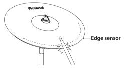
\* On the CY-13R, edge shots are possible when the connection is made to the BOW/EDGE OUTPUT jack.
