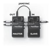
To use JamSync, connect the master JamMan Solo HD's **JAMSYNC OUT** jack to the **JAMSYNC IN** jack of the first slave device. Daisy chain any remaining JamSync slaves in the same manner.
